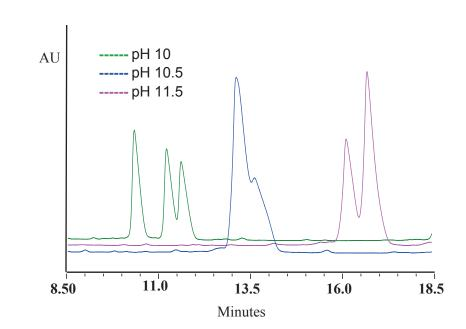
Figure 3. influence of mobile phase pH on resolution of oligonucleotides in anion-exchange chromatography (column: DNAPAK PA200, 250 x 4.0 mm, 8u; elution agent: sodium bromide)
