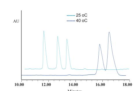
Figure 2B. Influence of column temperature on resolution of ologonucleotides in anion-exchange chromatography (column: DNA PAK PA200, 250 x 4.0 mm, 8u; elution agent: sodium bromide, pH 11.5)
