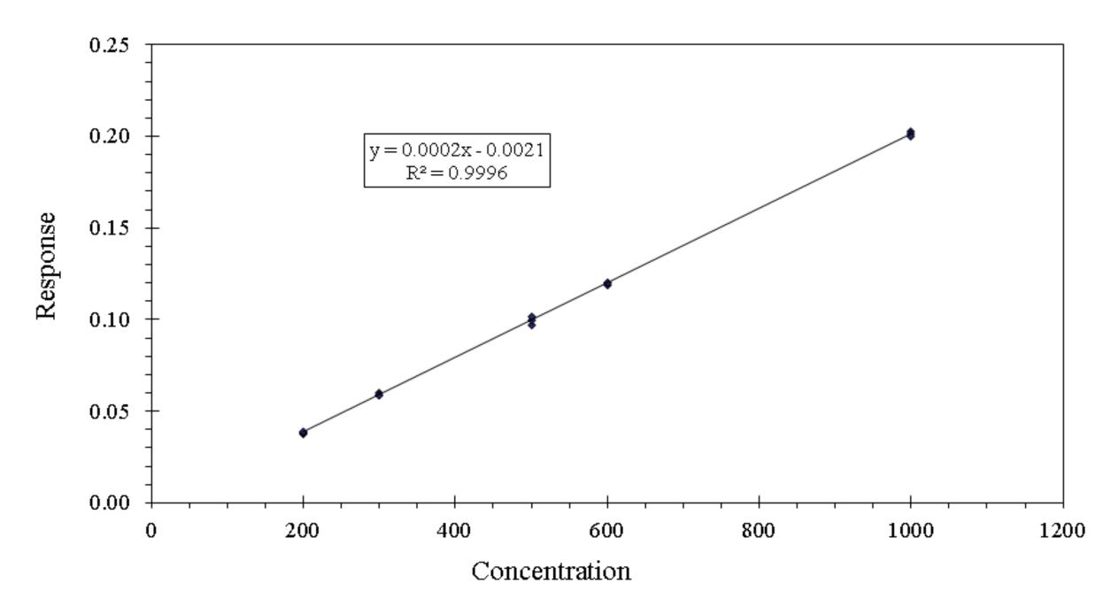
Figure 3: Calibration curve for atomic absorption standards
