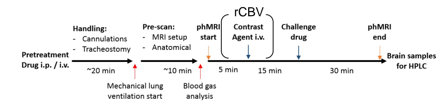
Figure 2. Example of phMRI experiment timeline. Contast injection is used only for rCBV measurements.
